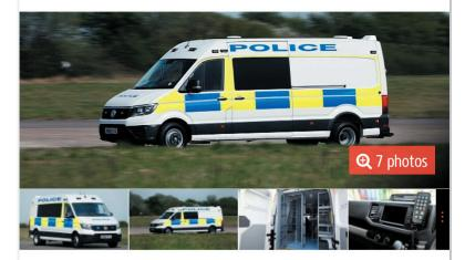
If you were wondering, "unbreakable" is Volkswagen for polycarbonate plastic resin. More to the point, the windshield is made of KASIGLAS marprotect material. In addition to seating for seven people in the rear and the half-width prison cell, the Crafter Police Support Unit also comes with a storage system designed to store riot helmets, shields, and various other equipment.
